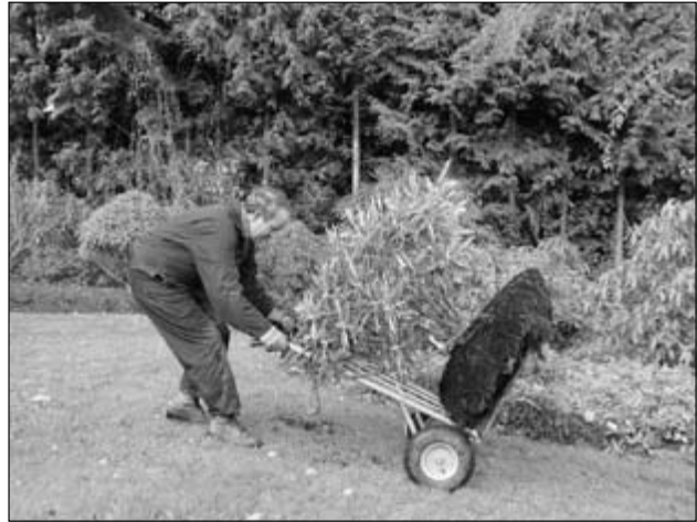
To balance the weight over the wheels, the handle must be kept at a low angle .
